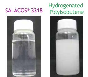
Figure 1. This image shows good compatibility of SALACOS® 3318 with silicone (30 cs) versus a competing material such as hydrogenated polyisobutene
