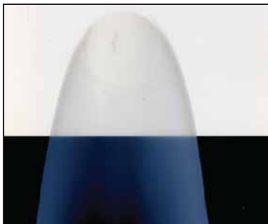
Drawdown of Dispersion (TiO 2 TA-100 in an Ester)
