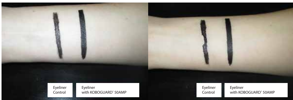
Pictures of Eyeliner Control and Eyeliner with Koboguard® 50AMP comparison of before (left) and after 15 wipes under running water (right)
