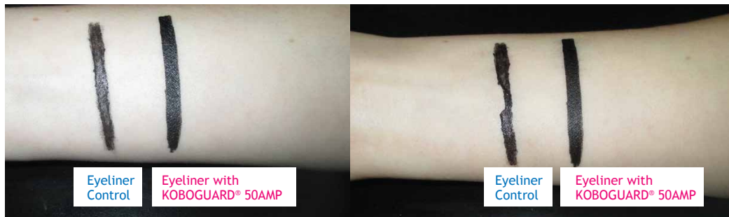
Pictures of Eyeliner Control and Eyeliner with Koboguard® 50AMP comparison of before (left) and after 15 wipes under running water (right)
