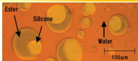
Figure 1. An image showing the possibility to emulsify insoluble oil combinations with large particle sizes
