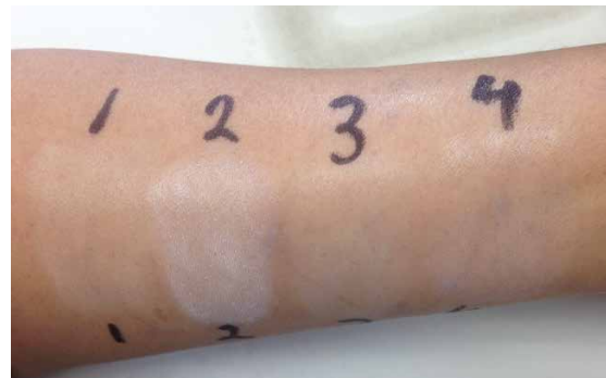
Skin whitening of IR blockers in formulation, compared to other titanium dioxides. At 5% in an emulsion, both IR blockers (1 and 3) are less whitening than Pigmentary \text{TiO}_2 (2) and similar to UV-attenuation grade \text{TiO}_2 (4).
