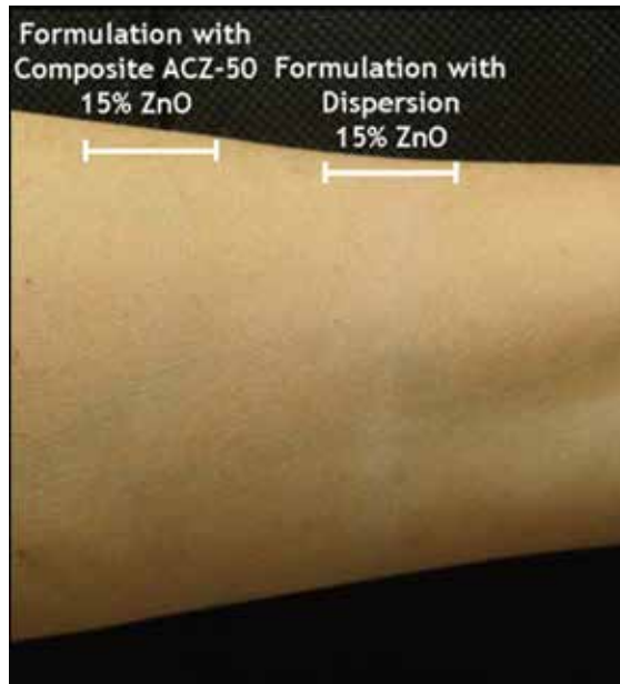
A comparison of a formulation containing COMPOSITE ACZ-50 and a formulation containing a traditional ZnO dispersion at a 15% concentration of ZnO applied on the skin
